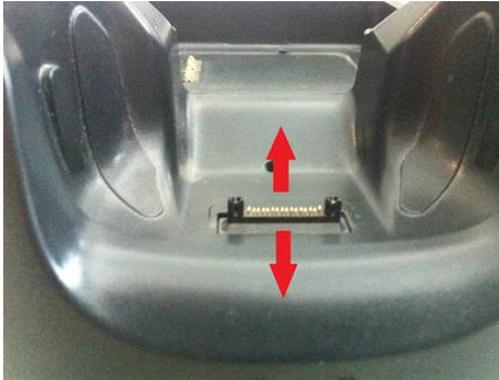
4. Use a dry cloth to remove any dirt near the contacts area and to clean the plastic parts. If the plastic parts of the equipment are very dirty, slightly dampen the cloth with only water.
