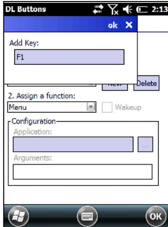
To assign a new function to the button, select the desired function and then tap 'OK':
