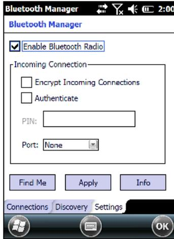
4. Tap ‘Find Me’ if you want to make the Skorpio X3 visible to other Bluetooth® devices for 60 seconds, allowing them to set up a connection.
