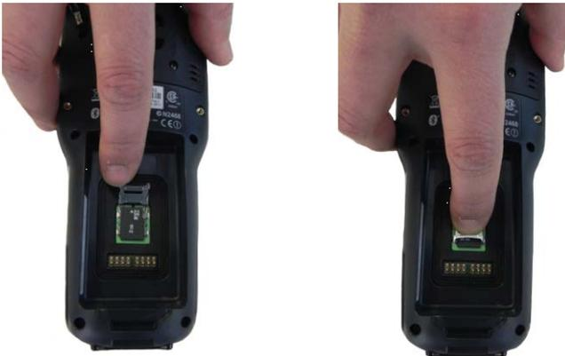
6. Insert the battery's alignment lugs into the recesses, then press firmly until the battery latch clicks twice.
