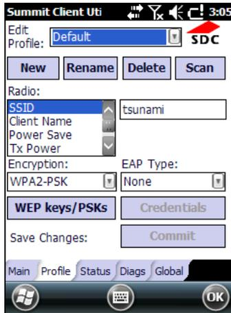
Information about the wireless network can be entered directly in the profile tab or by pressing "Scan" when the desired network SSID is in range.
