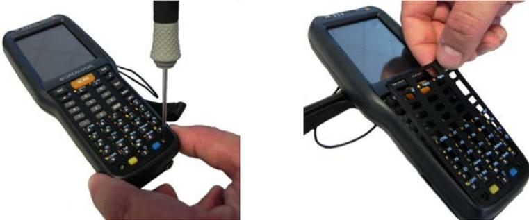
2. Insert the terminal emulation overlay (first the upper side):
