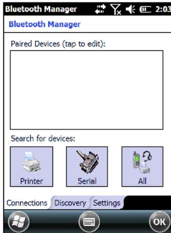
2. Search for available Bluetooth® devices by tapping the button for the type of device you want (Printer, Serial or All) or tap the Discovery tab and then tap the Discover button to skip this step. The Skorpio X3 will search for Bluetooth® devices within range.
