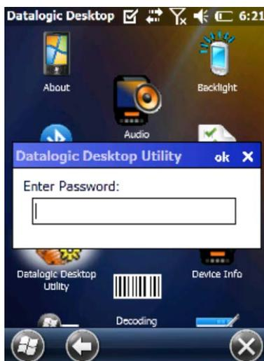
1. Type in your password using either the keypad on the unit, or using the stylus on the soft input panel (SIP).
