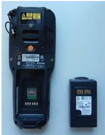
4. Insert the battery's alignment lugs into the recesses, then press firmly until the battery latch clicks twice:
