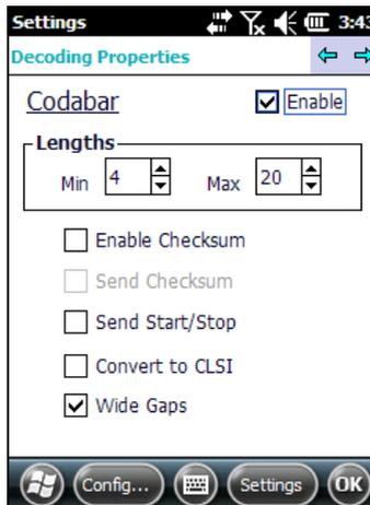
Codabar: Select Enable, Min/Max Lengths, Enable Checksum, Send Checksum, Send Start/Stop, Convert to CLSI and Wide Gaps.
