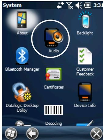
The audio control panel can be used to independently set the playback or recording volume for different types of audio inputs and outputs, such as a headset, powered mobile dock, or the internal speakers and microphone.
