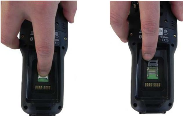
4. Insert the microSD card with the written part upward:
