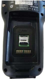
5. Lock the card into place by pushing the cardholder down and then shifting it downwards:
